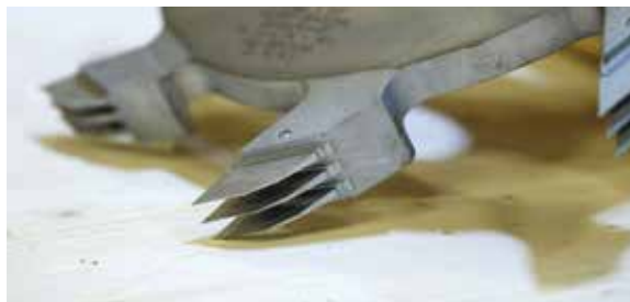
The geometry of the fingers was redesigned to provide more options for adjustment
