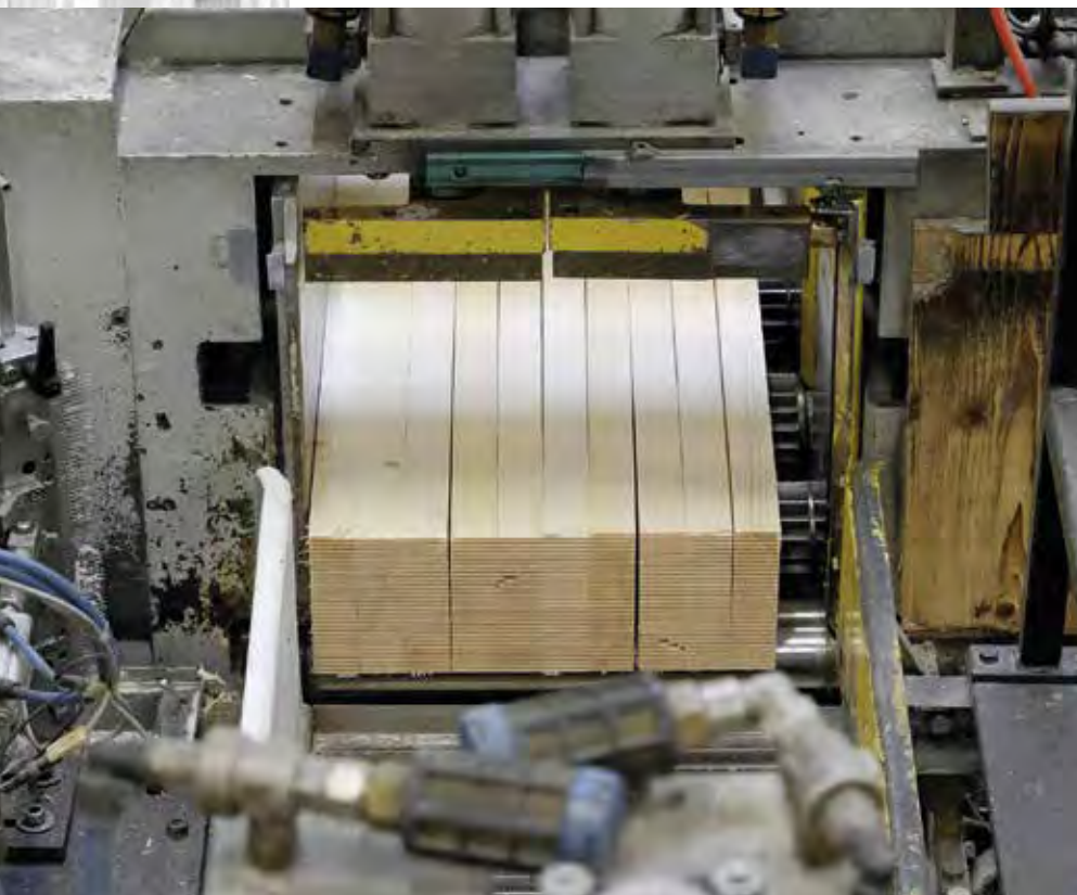
| The wider the individual lamella, the higher the cutting pressure.
