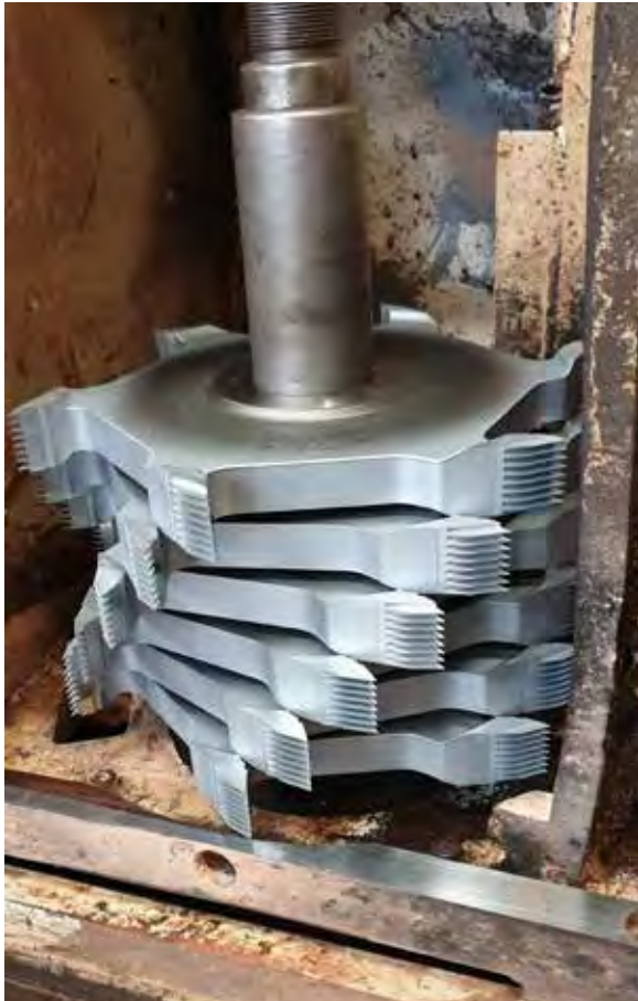
For up to 3 times longer tool lives LEUCO offers the micro finger jointing cutters with "LEUCO TOPCOAT" coating.
