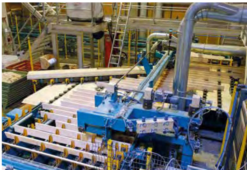
In the through-feed equipment, the fingers are cut at high speed
