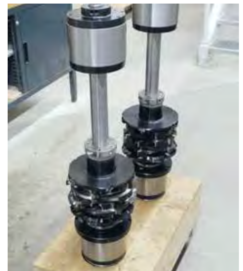
| Change shafts of the planer fitted with Vario 100 tool sets. A block height of up to 300 mm can be machined.
