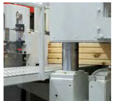
| With two vertical shafts, the planer can process profiles in one go.
