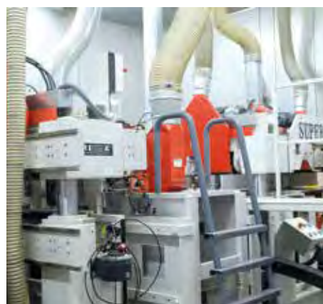
| The line dresses the sides, then profiles and planes the top and bottom.
