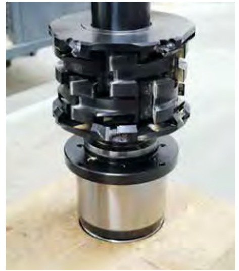
Tolerances of a few thousandths allow the high rotational accuracy, which results in a very nice surface quality of the milled logs produced.
