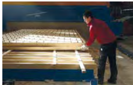
The work on the portal machining center from Hundegger was improved using the “LEUCO surfCut” by woodworker Rolf Rombach. His customers now demand an outstanding surface quality. Plain milling the elements is such a basic working step that now takes less time using the new tool, Tobias Wehrle shown here.
