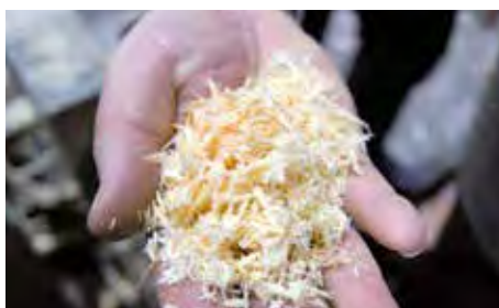
Shavings come from the profile cutter this fine and are collected separately
