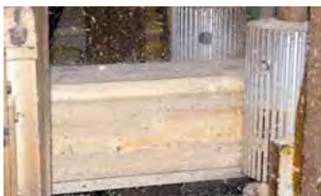
The tool works its way through the center wood at up to 75 m/min leaving a squeaky clean edge
