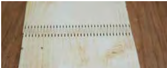
Clean fingers with a better fit were the result of the optimizations
