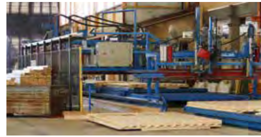
Cut-outs for windows and doors are taken into account when laying the boards and only have to be milled to a finish later on. Because each time the plain milling cutter moves back and forth and chipping occurs with and against the feed, the tool goes in and out of the edges numerous times. With the LEUCO “surfCut”, Rombach can operate the machine with 75% of its potential feed speed.
