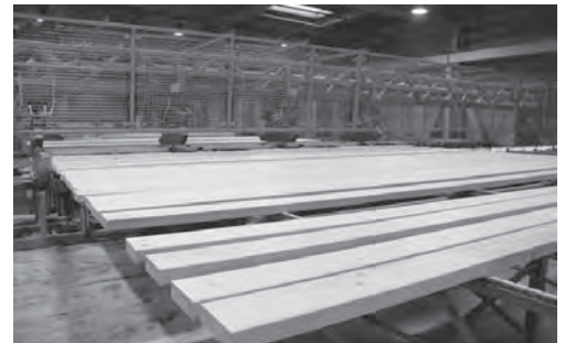
After planing, the quality laminated timber is cut to the desired length.
